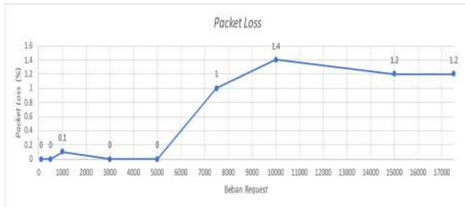
Figure 12. Graph of packet loss parameters in QoS testing
