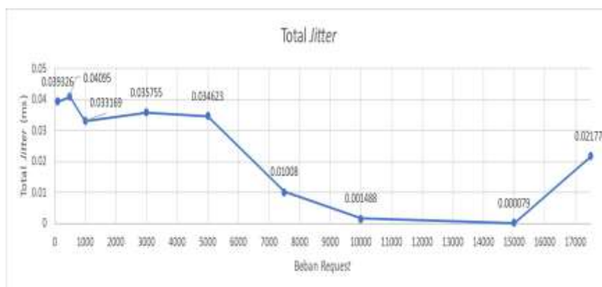
Figure 14. Graph of total jitter parameters in QoS testing
