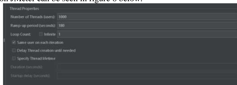
Figure 6. Test scenario settings on JMeter
