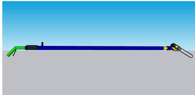
Figure 6. The portable oil palm harvester is shown right.
