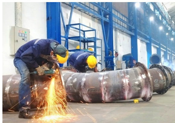
Figure 3: Grinding and finishing of welded Coal Pipe edges
