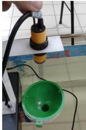
Figure 4.7 Image of the E18-D80NK Infrared Proximity Sensor in No Feed Conditions
