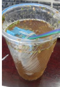
Figure 4.10 Sensor Testing in Turbid Water
