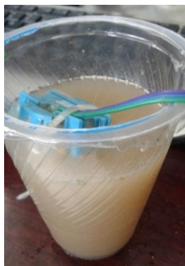
Figure 4.11 Sensor Testing in Very Turbid Water
