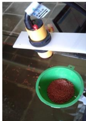
Figure 4.8 Image of the E18-D80NK Infrared Proximity Sensor in the Condition of Feed
